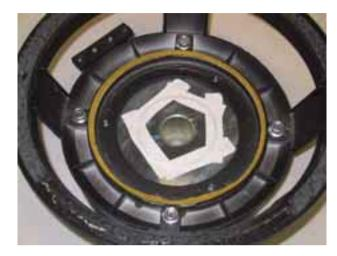
• Clean the magnet air gap using double face adhesive tape, the tape over the gap to keep any dirt from entering.
