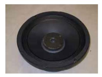
• Remove the plastic shims, glue the dust cap in place and solder the lead wires to terminals.
