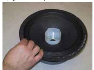
• Glue the gaskets in place and line up with the chassis holes. You can use the same glue as above or a vinyl type.
