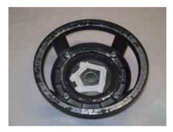
• Using a sharp tool, scrape away the glue particles from the chassis, where the surround and the spider were glued.
