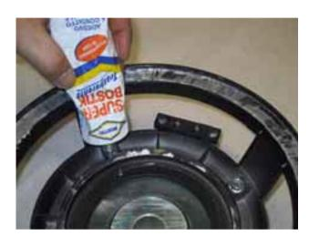
• Distribute the glue (either a two-component epoxy or a rubber type) on the cleaned chassis where the surround and the spider fit.
