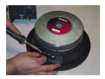
• Remove gaskets and unsolder the lead wires from terminals.
