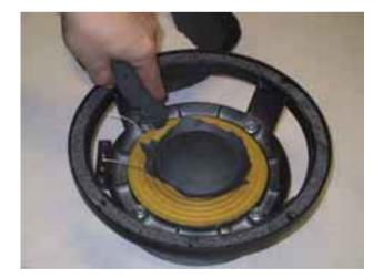
• Cut around the surround of cone and the spider and remove the cone.
