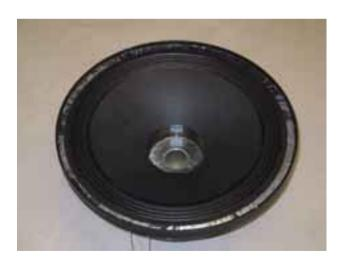
• Place the new cone assembly in the chassis, making sure the lead wires are in proximity of terminals.
